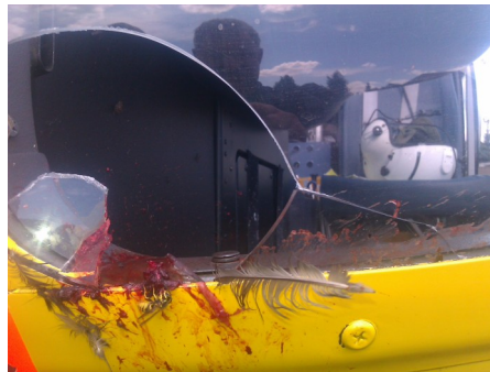
Helicopter windshield hit by a bird
